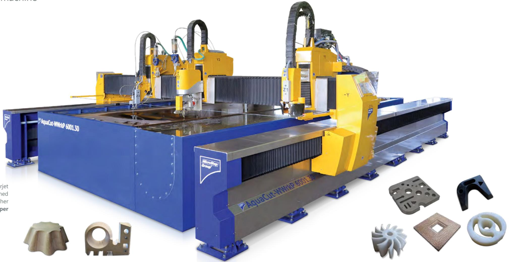
The **AquaCut** is a highly precise CNC waterjet cutting machine designed to process a wide variety of materials including those that cannot be subject to thermal or mechanical stresses.
