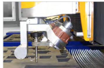
In order to meet the requirements for high precision and/or perpendicularity of the cut parts, MicroStep's Adaptive Bevel Compensation (ABC) technology enables taper compensation in a range of  $\pm 7^\circ$ . The technology adjusts the bevel angles with speed to compensate the natural stream lag and taper of a water jet. The system also allows custom adjustment of the compensation values.
