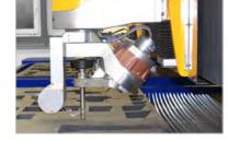
In order to meet the requirements for high precision and/or perpendicularity of the cut parts, MicroStep's Adaptive Bevel Compensation (ABC) technology enables taper compensation in a range of  $\pm$  7°. The technology adjusts the bevel angles with speed to compensate the natural stream lag and taper of a water jet. The system also allows custom adjustment of the compensation values.
