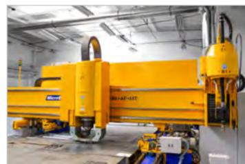
The DS series offers a variety of automated processing options for flat materials. Besides drilling, straight cutting and bevel cutting for weld edge preparation up to 50°, oxyfuel cutting, tapping, countersinking as well as scanning and marking are possible. The standard work area size is up to 6,000 x 2,000 mm.
