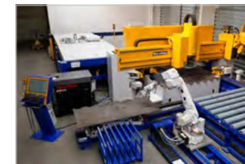
As a time- and cost-efficient production solution, the DS series has a high degree of automation. Loading of plates into the cutting zone, unloading of processed parts as well as separation of residual material are fully automated. The modular design of the machine allows to customize the unloading process incl. sorting by robots. Moreover, the machine is operated by MicroStep's production management software CyberFab® Manager that can be interconnected with local ERP system.
