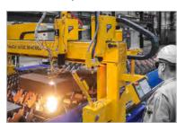
EasyCut machines are designed to withstand high workloads in multiple-shift operations including multi-torch parallel oxyfuel cutting of material thicknesses up to 300 mm. Intelligent temperature management keeps the system from exceeding its limits even in harsh environmental conditions and under intensive cutting load.
