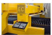
A standalone, ergonomic MMI console provides the operator with an overview of all cutting processes, machine related information as well as extensive multi-tasking features. Additionally, a handy operational panel on the gantry allows the operator to perform basic tasks suc as interrupt a cutting program, initialize or move the machine or perform a manual cut.
