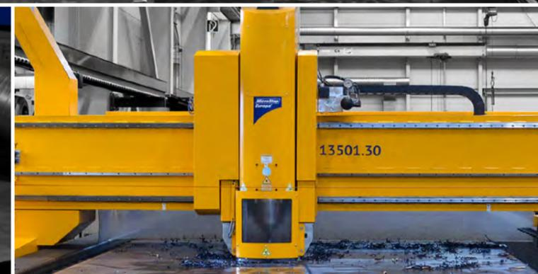
DRM's automatic drilling solution with 55 kW spindle with inner cooling and a dedicated drilling table
