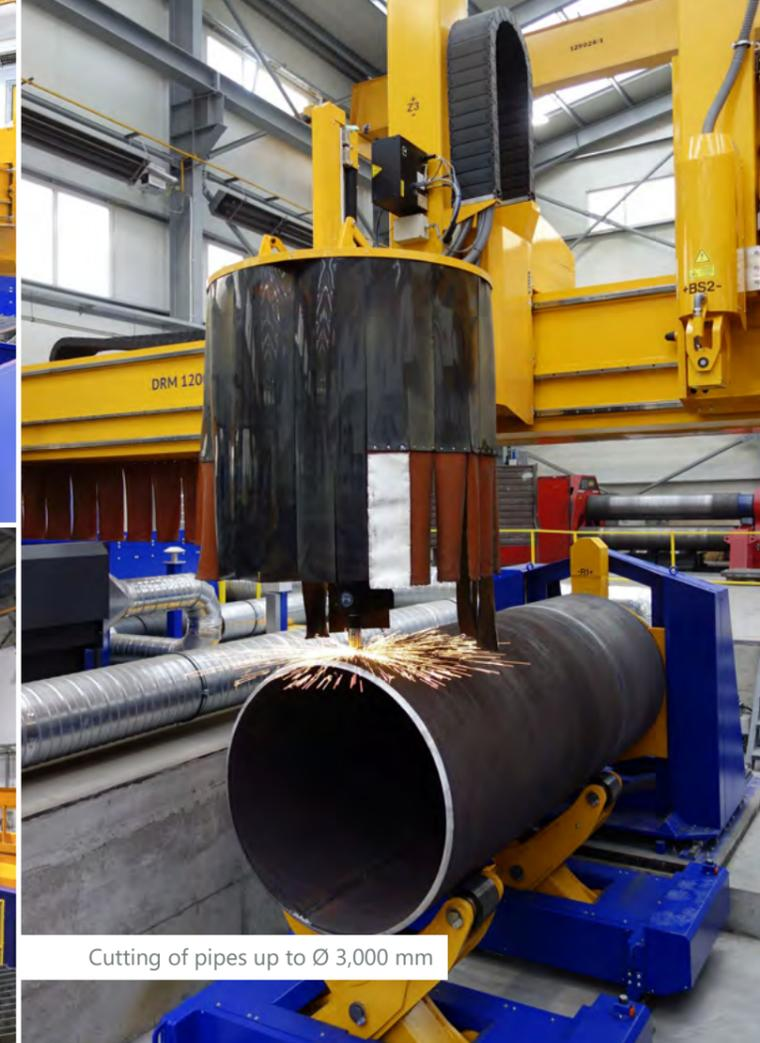
Cutting of pipes up to Ø 3,000 mm
