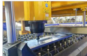
The powerful spindle enables drilling up to Ø 70 mm and a variety of milling operations such as large hole milling, face milling, pocket & slot milling, chamfer milling, thread milling or counter boring.
