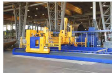
DRM Max can handle it all: in addition to its drilling and milling capabilities, the machine provides all the advanced functionalities of other MicroStep cutting machines, such as bevel cutting, tapping, countersinking, marking and scanning.
