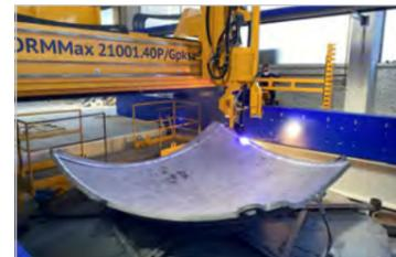
DRM Max can process a whole range of workpieces including domes up to a height of 1,500 mm as well as dome petals. A 3D laser scanner and mScan technology compensate for possible deviations of the real domes for achieving outstanding precision.
