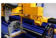
MSF Pipe machines are equipped with a 3D laser scanner that scans the exact shape of the workpiece in the place of cutting. Advanced algorithms then allow the control system to adjust the movement of cutting tool and pipe supports accordingly and compensate for possible inaccuracies of the particular pipe or
