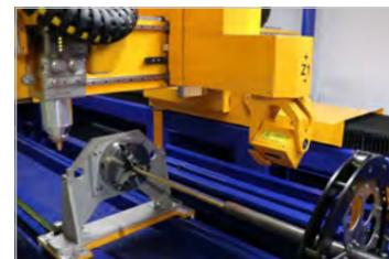
MSF Pipe machines are equipped with a 3D laser scanner that scans the exact shape of the workpiece in the place of cutting. Advanced algorithms then allow the control system to adjust the movement of cutting tool and pipe supports accordingly and compensate for possible inaccuracies of the particular pipe or profile.
