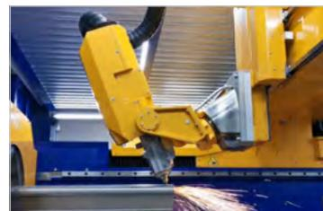
MSF Pipe can process pipes and profiles with different cross-sections: from common round and elliptical pipes through square and rectangular hollow profiles to special shaped profiles.
