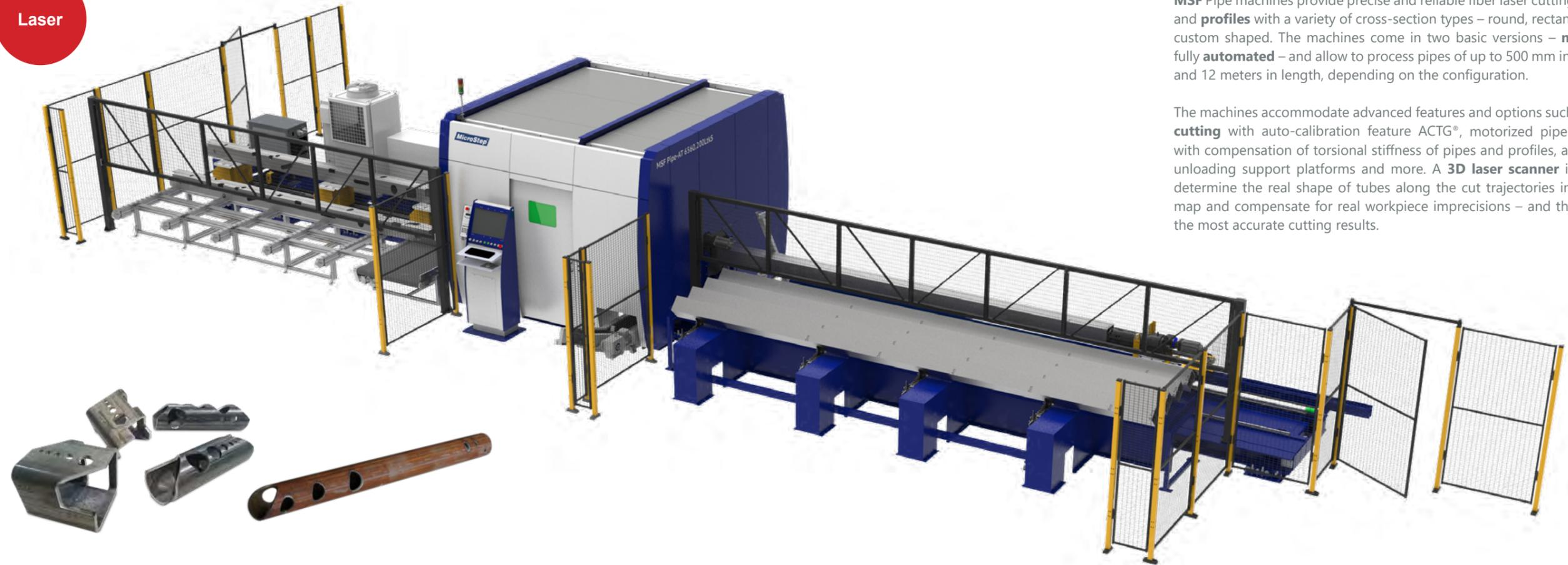
**MSF Pipe** machines provide precise and reliable fiber laser cutting of **pipes** and **profiles** with a variety of cross-section types – round, rectangular and custom shaped. The machines come in two basic versions – **manual** or fully **automated** – and allow to process pipes of up to 500 mm in diameter and 12 meters in length, depending on the configuration.
