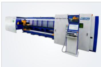
For applications with less workload or a tight floor plan, a version of MSF Pipe with manual loading and unloading is available. The machine features motorized pipe supports that enable convenient positioning and a smooth, efficient cutting process. Torsional stiffness compensation is provided for pipes with smaller diameters.
