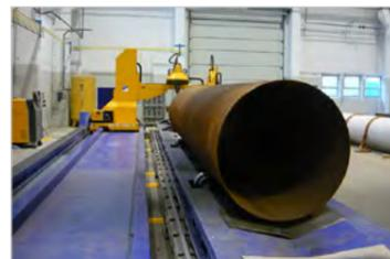
Thanks to the open machine area with low-positioned guidelines in the longitudinal axis and the mobile cantilever gantry construction, the gantry can be parked aside to ensure convenient and safe loading and unloading even for large pipes and profiles.
