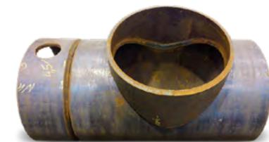
3D pipe and profile cutting up to Ø 2,000 mm
