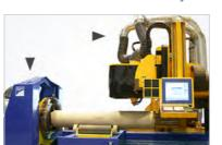
MicroStep's proven suction design for pipe cutting includes direct fume extraction from inside of the pipe through chuck as well as suction from the overhead cover around the cutting head.
