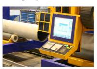
A control unit with touchscreen mounted on the gantry provides all positioning and technology control functions and thus ensures convenient operation of the machine along its whole length.
