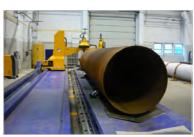
Thanks to the open machine area with low-positioned guidelines in the longitudinal axis and the mobile cantilever gantry construction, the gantry can be parked aside to ensure convenient and safe loading and unloading even for large pipes and profiles.
